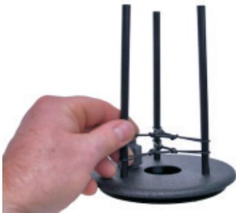
assemblies away from the Front Plate and insert your microphone into them. You can use your microphone pointed towards the dish, recommended, or away from the dish. Align your microphone so that the element of the mic is exactly 3 13/16 or 97mm from the surface of the Front Plate. Connect
