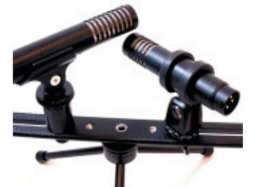
The picture on the left shows how a quick release tripod mount, camera, and recorder can all be mounted. The picture on the right shows a typical XY microphone configuration, using the Spacer to lift one mic above the other.
