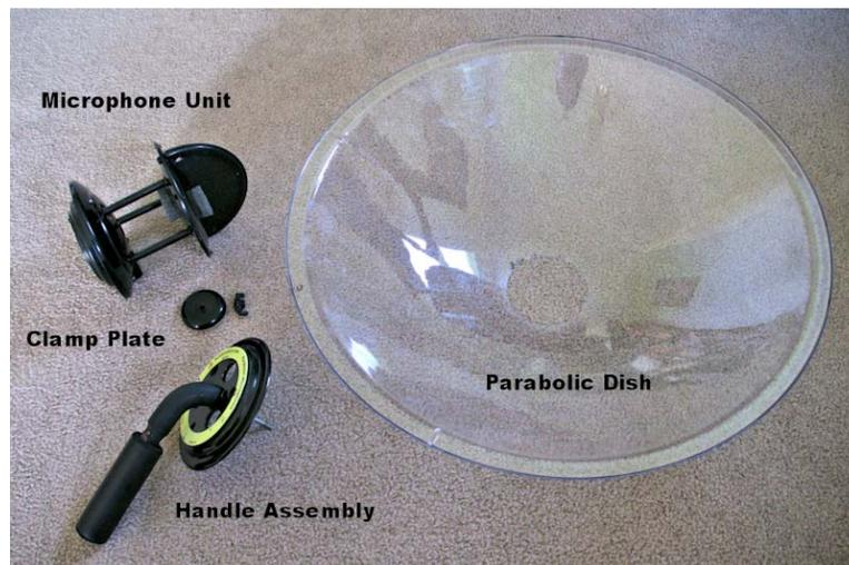
*Major components of the parabolic microphone.*
