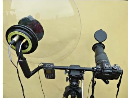
*Mount cameras and recorders to tripod.*
