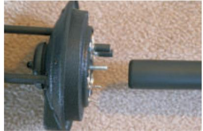
Showing how the Mic Unit stud can be threaded into the Handle Base.
