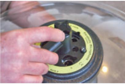
Align and slightly tighten knob.
