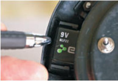
Pry up on battery to remove.
